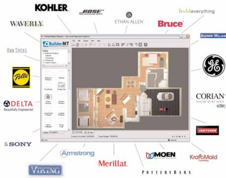
This CAD-based, virtual "plan view" of a typical residence is accompanied by a sidebar that contains product folders of potential product providers. Inside each folder are products that users can drag and drop into the image. Product specs and procurement data are captured as selections are made.
